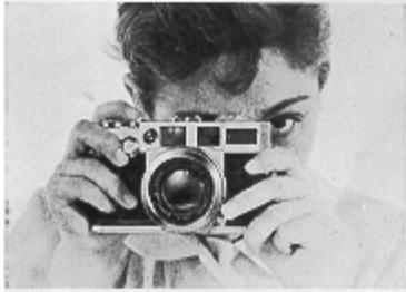
Hold the camera in both hands using the right index finger to operate the shutter release and left index or middle finger to adjust focusing. When using telephoto lens it is advisable to turn the lens barrel instead of focusing knob. To look through the viewfinder either the left or the right eye will do. Use whichever is convenient to you. Stabilize the camera by holding it so that the left hand thumb is pressed against your cheek.
