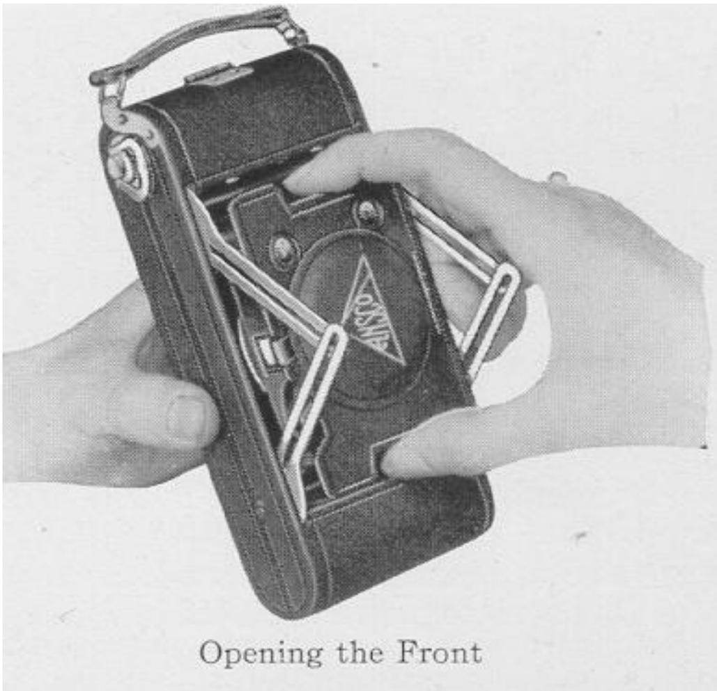
Holding the camera in the left hand, draw out the bellows with the thumb and middle finger of the right hand. When full extension is reached, the side arms will snap into place, automatically locking the front at that point. Open the watch-cover lid that protects the lens by releasing the spring snap at the top of the camera. Attach the wire release by threading it into the socket provided for it, which will be found beside the finger release. The ANSCO is then ready for focusing on the subject.
