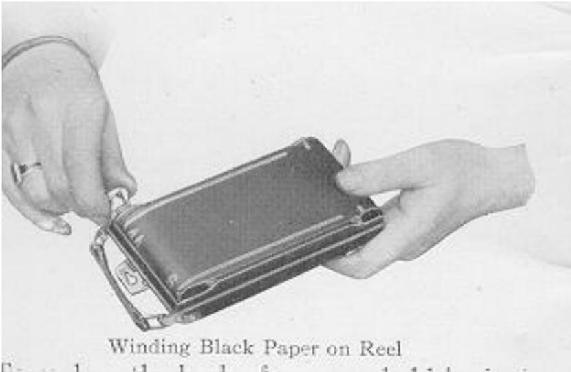
To replace the back of camera, hold its body with the left hand, and with the right hand hook the back on the dowels at one end, then close down and fasten the hinged catch. Next, turn winding key to the right until the figure 1 appears in front of the little ruby window.
