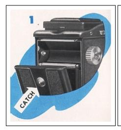
Open the back of the camera by pressing down on the locking catch. The back is hinged for convenience. Hold camera so back does not drop or hinge may be sprung.
