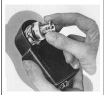
When using midget flash bulbs, use the adapter. It is a permanent part of the unit when attached. The Flash Unit Reflector is readily removable ... should be adjusted so center of bulb is 1" from back of curved section. Lacquer coated. Clean only with a damp cloth.
