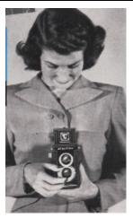
To focus the Argoflex, open the focusing hood, using the right thumb, as shown.
