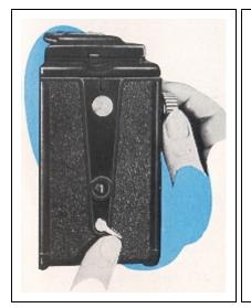
Hold lever on back of camera, using left thumb, and wind until Figure 1 appears in the center of the red window. Do not wind beyond this point.
