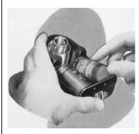
The front part of the battery case is removable. Hold the unit in the left hand and pull off cover with right hand.
