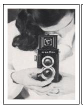
Hold the camera in the manner illustrated, and focus by turning the knurled lens mount until the ground glass image is sharp.
