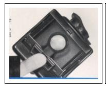
For critically sharp focusing, use the magnifier. Using the thumb, flip it into position as indicated by the illustration.
