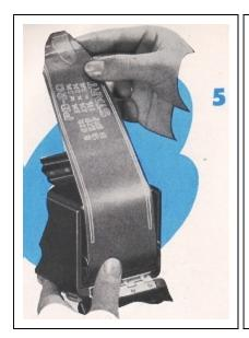
Holding cradle in with the left hand, pull off about 8 inches of paper leader for threading.
