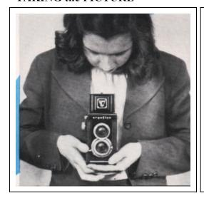
To take the picture, hold the camera as shown, and compose the subject on the ground glass as you want it to appear in the finished picture. A lower or higher position may be desirable to get just the effect you want. Then, hold your breath for an instant and press the shutter release SMOOTHLY with the right thumb. Take care not to jar the camera or the picture may be blurred due to camera movement.
