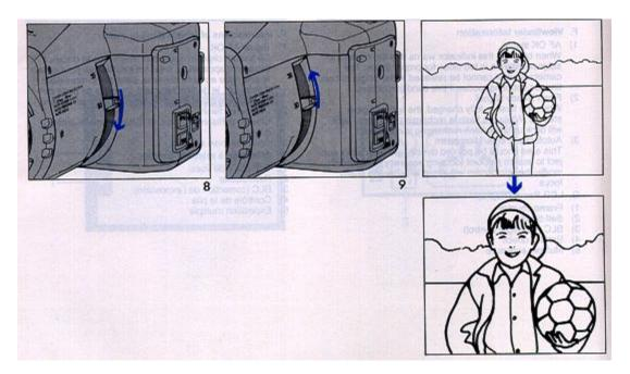
1) Telephotography When a telephoto perspective is desired, move the zoom lever in the direction of the tele (80 mm) position. (Fig. 8)
