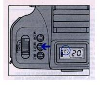
The self-timer can be cancelled by pressing the self-timer button again or by setting the main switch to "OFF".
