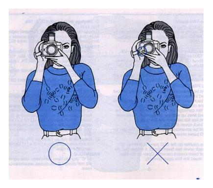
Hold the camera so that fingers carrying straps, etc. will not cover any part of the flash unit, lens, or the AF measuring windows.
