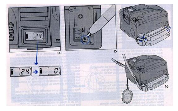
1 ) When the entire film cassette has been used, the film will automatically start to rewind within two to three seconds. (Fig. 14)
