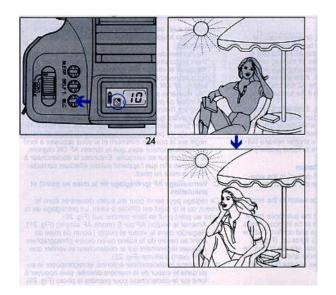
When the backlight control (BLC) button is pressed, the BLC indicator will appear in the LCD panel. When the shutter release button is depressed the exposure will be corrected automatically. (Fig. 24)
