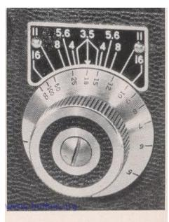
The Ciro-flex Depth-of-Focus Scale is located on the camerabody just above the focusing knob. To use this scale, focus the camera as already explained or simply judge the distance between the camera lens and your subject.
