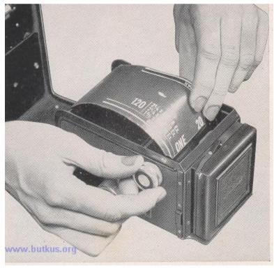
To give film maximum protection from light, window should be kept closed at all times except when transporting film to next exposure number.
