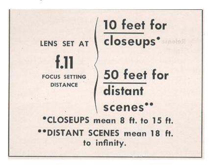
When taking ordinary snapshots, it is not always necessary to focus on the ground glass. By merely using the depth-of-focus scale, you can readily "set" your camera for a "zone of sharpness" and follow this famous Ciroflex snapshot rule:
