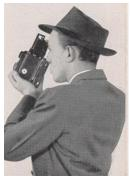
The Ciro-flex Sportsfinder is a small opening in the back panel of the viewing hood to serve your need for fast-action sports shots. For sharper, clearer action prints, pre-focus on the ground glass as described above using some object where the action is to occur as your focal point.
