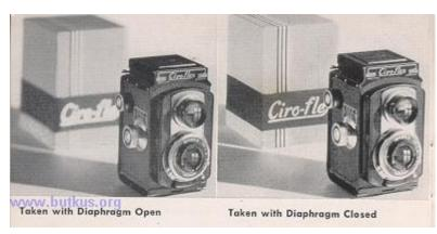
When the lens is focused on a point or object, those subjects somewhat nearer and farther away from the lens are relatively sharp also. This effect is called "depth-of-focus". As the diaphragm is made smaller . . . i.e., as the lens is stepped down, you will note that this field of relatively sharp focus is extended to subjects even nearer and farther away from the object upon which the lens is focused as illustrated above.
