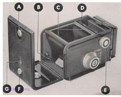
Open the camera by pressing down on *Button A* and lifting out on back cover panel.
