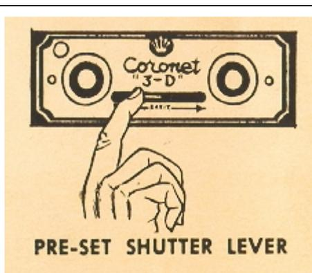
Set the shutter by moving the preset lever on the face of the camera. Hold the camera up to your eyes. Your Coronet 3-D camera has a binocular-type viewfinder allowing the use of both eyes for maximum comfort and accurate 3-D composition. Hold the camera at level with subject and steady.
