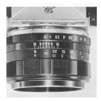
2. The depth of field Scale on the lens barrel lets you know the depth of field of the lens in use. If the subject is at a distance of 3.5 feet and the aperture setting is set at f/16, all objects within the range indicated by the figure 16 on both sides of the red index (approx. 3.1 feet to 4 feet) will appear clear in the picture (in case of f/1.8 lens.
