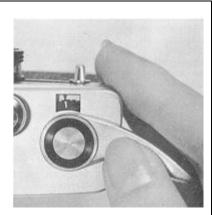
5. Advance the film by alternately winding on and depressing the Shutter Release Button until the Exposure Counter indicates the figure "1". You are then ready to shoot your first shot. The Exposure Counter shows you the number of the exposed frames.
