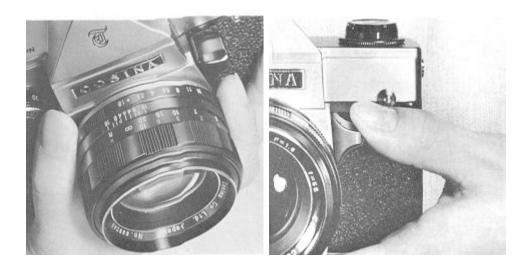
The diaphragm is stopped down to the preselected aperture setting for measuring exposure at the taking aperture.
