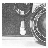
3. The Self-Timer functions when the Shutter Release Button is depressed, and trips the shutter by delayed-action after 8 seconds.
