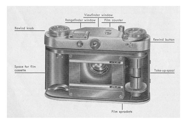
Loading the camera Is simple and can be done extremely Fast. Detailed instructions are given in the corresponding chapters of this booklet. Since this is a precision instrument, we urge you to study the instructions carefully before using your camera. We recommend that You make a couple of tests with a roll of film
