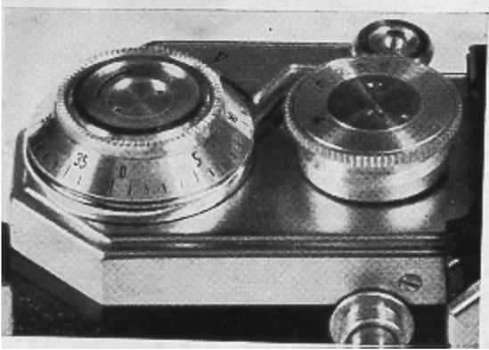
The indicator (exposure marker) is the triangle engraved on the lever (8). Pre shutter release button (9). Make two blank exposures by winding lever and pressing shutter release button. The exposure counter will point to exposure No. 1, and the camera is ready for your first picture. You can be sure that the film transports in your camera properly if the rewind knob (3) turns counter clockwise as you turn the lever (8) to the right.
