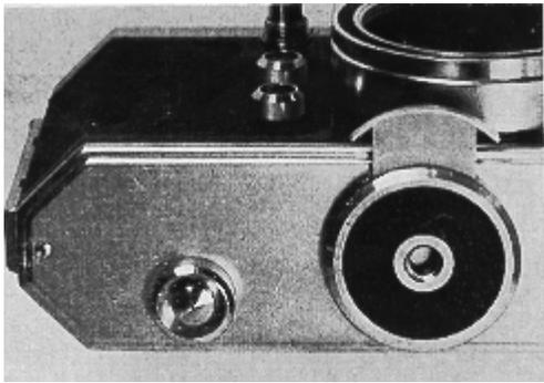
After all the pictures have been taken, the film must be rewound into the original cartridge. This is done by pressing down on the button (26) located on the bottom of the camera, and at the same time turning the rewind Knob (3) clockwise (to the right). As long as film is still in the camera, you will feel the effort of winding, which stops as soon as all the film is back in the cartridge.
