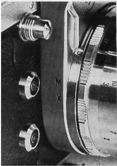
The EDIXA-Reflex is fully synchronized for regular flashbulbs and electronic flash. On the front of the camera are two contact sockets. The top socket (marked M on the side of the lens mount) is used for flashbulbs. The bottom socket (marked X) is used for strobe and electronic flash .
