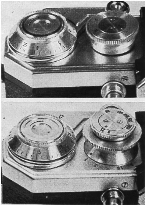
The speeds are set by means of adjusting knob (17) and the Knob (18). The engraved figures on the Knobs (17) and (18) indicate fractions of seconds: for example, 50 means 1/50 of a second, 5 means 1/5 of a second etc.
