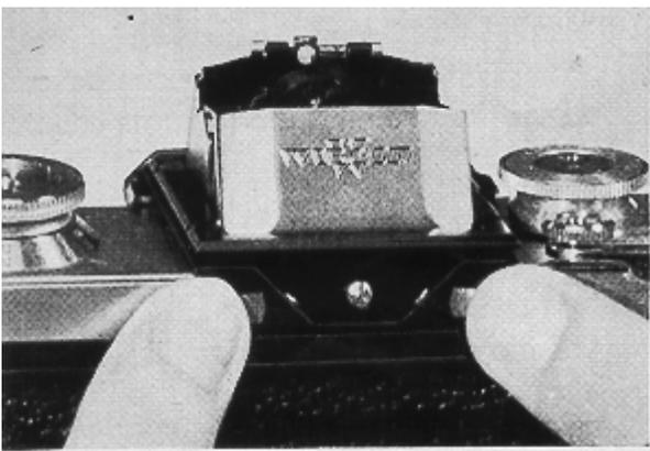
Press the small button on the back of the finder (on back of camera) and it will open automatically. To close, just press down any of the walls of the finder till the cat clicks. To bring the magnifying lens into position, press the small lever next to the lens. The image viewed on the ground glass (after you wind the shutter) will be reproduced on film, in the same size. As you turn the focusing ring on the lens, the image on the ground glass changes.
