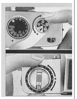
will be opposite the orange-colored triangles. On the filmsensitivity reminder disc (15) the figures from 9 to 33 are DIN values, whereas the figures from 6 to 1600 denote ASA values. The film-type symbols on the reminder disc (8) have the following meaning:
