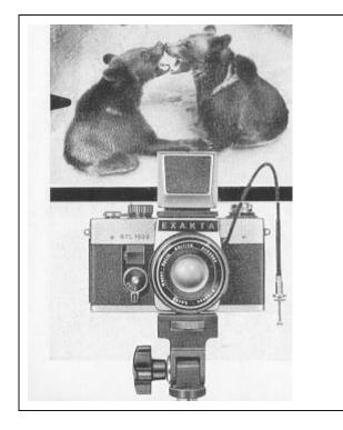
2. The image in any of the viewfinder systems (Finder Hood, Penta Prism, and TTL Penta Prism) will be visible even after the shutter has been released (instant return mirror). The red warning signal in the image in the viewfinder system indicates that the camera is not yet ready for action, and that the rapid-wind lever (9) must be wound before the shutter is ready for release (See illustration: image seen through the Penta Prism).
