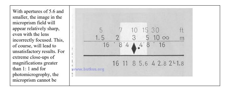
used. The rest of the image in the viewfinder (Fresnel field) does not serve for focusing the lens.
