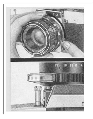
Changing the lens (22) : Press the locking lever (19) towards the lens. Then turn the lens to the left until the orange-colored dots (12 and 13) ore in line. Lift the lens out towards the front, -- To insert a lens, proceed in the reverse sequence: line up the orange-colored dots, and turn the lens to the right until it locks in place.
