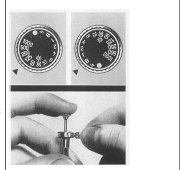
For working with the B setting a cable release with time-exposure lock can be recommended: After depressing the cable release, operate the time exposure lock. The shutter will remain opened without having to keep ones finger constantly on the release (also eliminating camera shake) until the time-exposure lock is disengaged.
