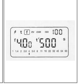
Note: The 1/10th stop values stored from the last measurement appear when the aperture is preset. These are invalid because the valid 1/10th stops will only appear after the next meter reading is taken.
