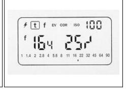
o The measured aperture stop appears on the left-hand digital display (resolution: 1/10th stops), and additionally as a mark rounded off in the analog aperture scale.
