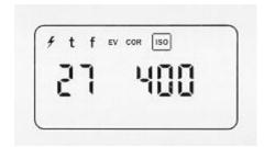
Once the film speed has been set it is transferred to the memory of the LUNA-STAR F when the meter is adjusted to any operating function, and it remains visible at the top on the right-hand side of the digital display. Any change of the film speed directly influences the stored paired aperture and shutter values.
