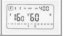
\* The measured aperture stop (from the sum total of flash and continuous light) appears on the left digital display, and as a flashing mark on the analog aperture scale. The aperture stop for the Share of continuous light is additionally indicated on the aperture scale (in our example f/8).
