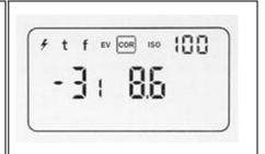
The extension factor appears on the right-hand digital display, the correction value is shown on the left in steps.
