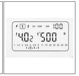
\* After the measuring button is released, the entire contrast range measured is indicated on the analog aperture scale. The last value measured does not flash any longer.
