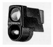
Reduces the measuring angle of your LUNASTAR F from 30° down to 5° for reflected light measurements and enables you to accurately frame in the viewfinder the part of the subject to be measured. The 5° SPOT Attachment is suitable for both ambient and flash light measurements:
