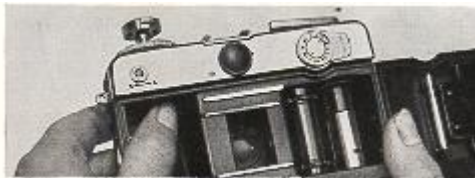
Before inserting film cartridge, push film spindle up
