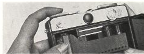
After inserting film cartridge, push film spindle down
