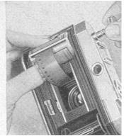
To open the camera, move locking slide outwards and swing the camera back open. Firm pressure on the camera back will help to release the locking slide.
