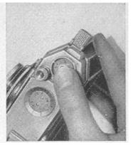
Insert flap of film in slit of spool up to second film perforation with which the carrying tooth must engage correctly. Turn milled disc of spool until the film is tightly stretched. The film must be pulled out of the cartridge in its full width by about 1/2" and must lie within the edges of the film channel. Then lower hinged film guide,
