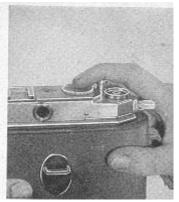
Press the brace-lock device which makes the lens board spring forward into position for taking pictures. At low temperature lens board may need a gentle pull.
