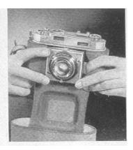
Set rapid-feeding lever once more, the counter disc now shows the number 1 and the first exposure can be made. Camera must be kept level. Hold it steady with both hands. Before making exposure check aperture and exposure time once more. When taking upright pictures, the little finger of the left hand holds back the lid of the Ever-ready case. There are three things to remember:
