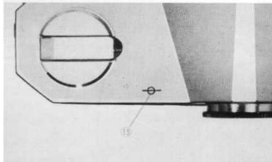
**Focal Plane Mark :** The distances shown on the Distance Scale 233 are those from the Focal Plane Mark "--" 15' which indicates the position of the film plane.
