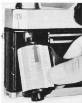
2 Direct toward the underside of the camera that side of the cartridge through which its spindle sticks out and put the cartridge into the Cartridge Chamber 2 .
