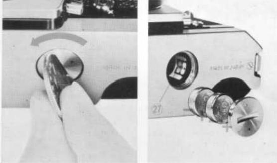
The compound CdS meter of the KONICA AUTOREFLEX A takes two 1.3V mercury battery cells as its electric source. Wipe the mercury battery cells, accessories for camera, with a piece of dry and clean cloth and put them into the mercury battery chamber.
