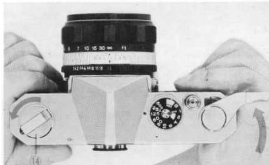
**To Check Film Advance:** When the film is being taken up in a correct manner, the Film Rewind Knob 14) turns counterclockwise. If it does not turn counterclockwise, it means that the film is not being properly wound. This manual was created by [www.butkus.org/chinon](http://www.butkus.org/chinon) and should only be found at my site.
