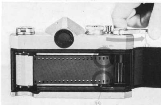
131 Insert the film tip into the Film Take-up Slit 33- of the Film Take-up Spool 341. Any slit is usable. Choose any slit into which the film tip can be inserted with ease.
