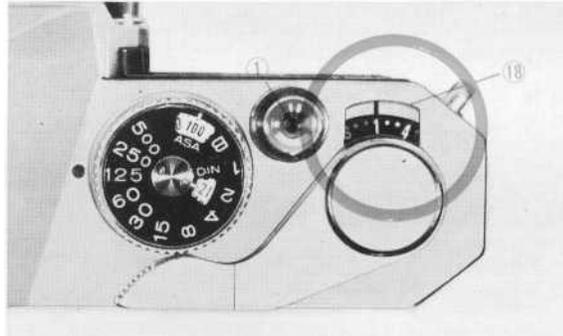
**F51** After the back cover is closed, flip up the Film Rewind Crank 13 and turn it in the direction indicated by an arrow mark on it to reduce the slack of the film.
