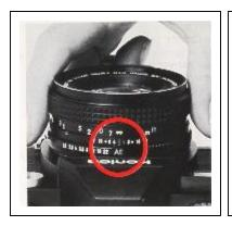
In AE Photography (Automatic Exposure) Turn the lens aperture ring to the AE mark. A safety lock will prevent accidental change.
