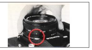
To remove the lens, hold the base of the lens and turn it counterclockwise, while the lens interchange button is kept depressed. Take out the lens when the red dot of the lens comes in line with the lens mount/dismount indicator of the camera body (red dot).
