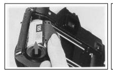
Insert the 35mm film cassette into the film chamber from the cutout lower section.
