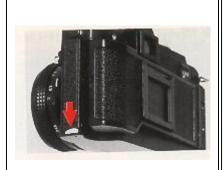
The Konica FS-1's autoload system is so designed that once the film is set to a prescribed position and the back cover closed, the film will be automatically transported by one frame. Film loading has been somewhat troublesome in the past, but your Konica FS-1 enables you to do it safely and surely.
