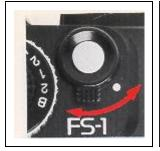
Move the lever around the shutter button till the white dot visible, and the shutter will be released. When the lever is alignment with the red dot, the shutter will be locked and the safety device to prevent an unnecessary depression of the shutter button will be activated.
