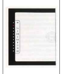
For stopped-down metering, look through the finder and turn the aperture ring or the shutter speed dial, while the shutter button is lightly depressed.
