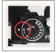
The B (bulb) exposure mechanism is used for an exposure of more than three seconds. Set the shutter speed dial to B and depress the shutter button, and the shutter will be opened. When the finger is detached from the button, the shutter will be closed. If your camera is set to manual and a desired shutter speed, a long-time exposure may be made.
