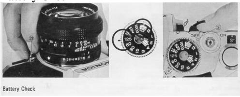
Remove lens by pressing Lens Lock Release Button (28) tuning lens as shown. Set film speed at ASA 100, shutter speed at 1/125th. Now, turn the Meter On/Off Switch (3) *past* the "Off" position to the engraved "C" (Check). If the Needle (51) in the viewfinder points to the Battery Test Indicator (52), your batteries are in good condition. Additionally, this also provides verification that the meter movement is correctly "zeroed" or aligned -- an extremely valuable feature.
