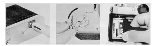
After all the pictures on the roll have been taken, the film is rewound into the cassette prior to removal for processing.
