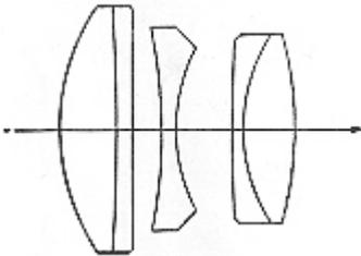
"HIGHKOR" LENS is designed for miniature negatives which are to be enlarged to huge proportions and yet are to retain in the completeness of the minutest detail. They are coated to reduce surface and internal reflections.
