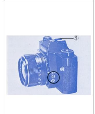
Your camera is provided with two flash Sync Terminals: FP for synchronization with FP class flash bulbs, and X for synchronization with electronic flash units. Compact electronic flash units designed for cordless operation may be attached to the Hot-Shoe (5) after its Safety Cover is removed. For a large flash unit used with a bracket, or for a compact electronic flash unit without provision for cordless operation, attach the flash synchronization cord to the appropriate Sync Terminal.
