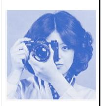
Support the camera in the palm of the left hand with the thumb and forefinger gripping the Focusing Ring. The palm of the right hand should fit against the right side of the camera body with the forefinger resting near the Shutter Release Button and the thumb on the camera back.
