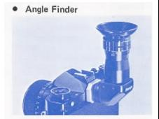
The Angle Finder is useful for low angles and copy work. The Angle Finder has click stops every 90°, but freely rotates a full 360° and has built in diopter corrections of--4 to +4.
