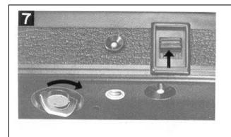
3. Turn the Attachment Screw Key to fasten the Winder to the camera. After turning on the Power Switch, the Mamiya Winder ZE is ready for use (Fig. 7).
