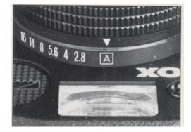
Program automation For all shots without flash set the white arrowhead on the lens mount (12) to A (automatic control).
