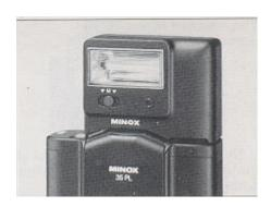
The Minox FC 35 electronic flash is the smaller of the two computer flashes designed for the Minox 35 cameras. It is 3 x 5.5 x 7.5 cm (1.2 x 2.2x3in.)1argeandweighs130g(4.6 oz). The metric guide No. for 100 ASA is 18 (59 in feet).
