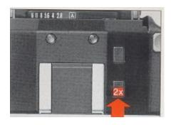
If you push the backlight switch (4) -the small rectangular button next to the hot shoe - fully forward, this automatically doubles the exposure.
