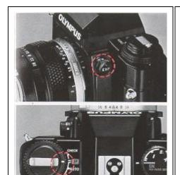
Make sure the camera is set for the ESP meter
