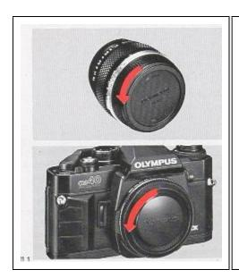
Remove the rear lens cap.
