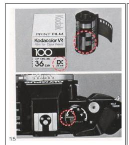
Make sure the film you are using is marked "DX". If the film you are using is not marked ""DX"" refer to page 31.
