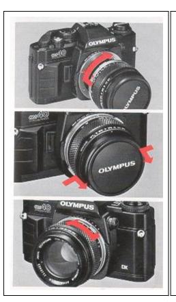
Align the red dots and rotate the lens clock wise until it locks.
