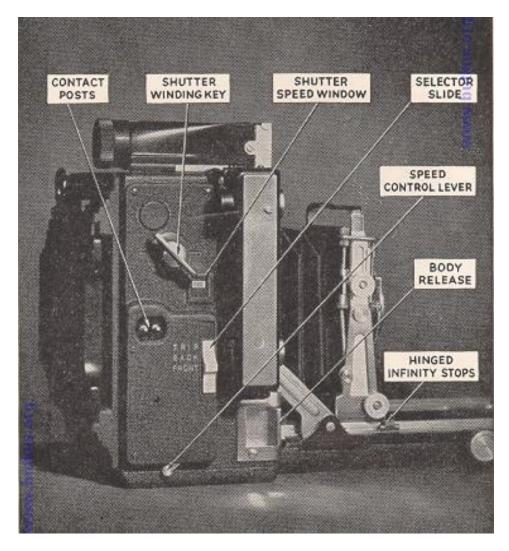
The Supermatic (X) Shutter is operated in the manner already described. The contact posts on the side of the shutter are intended to be used only with Class "X" (zero delay) high speed electronic flash units, and not with standard flash lamps. For synchronization with standard flash lamps, and relay operated high speed units, a solenoid should be attached to the shutter and synchronized with its operation.
