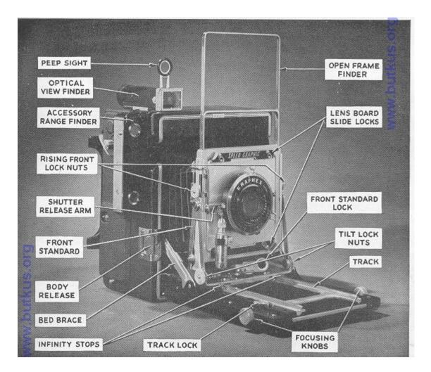
**Opening the Camera:** the bed release button located at the top center or top left side of the camera body. Draw the front standard out to the infinity stops and lock.
