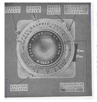
**Selecting Speeds:** Turn the outer knurled ring until a pointer is opposite the shutter speed number for the exposure required.
