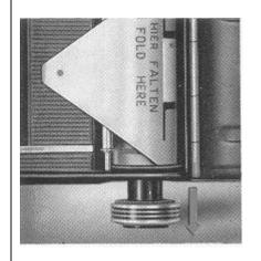
Now open the camera back, pull out the spool support and lock it in position. Tip the spool with the exposed film into your hand and fasten the paper trailer with the gumstrip. Should the camera be firmly connected to any other equipment the film spool can also be removed by means of its lower flange.
