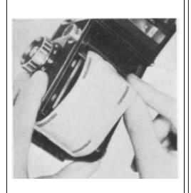
(**Note**: Make sure that the film is centered evenly on the take-up spool; otherwise it may climb on the end of the spool after the camera is closed and cause tearing of the paper).
