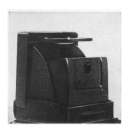
1. Magnifying Glass (17) is raised into position by pushing the upper edge of Eye-level View-finder Frame Plate (2) inwards. This will snap it into position. The eye should be brought as close as possible to Magnifying Glass (17) to obtain "hair-line" focusing.
