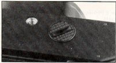
A close-up photograph of the battery compartment cover on a camera. A coin is being used to turn the cover counter-clockwise. The number '3' is printed in the bottom right corner of the image.                 | <p>1. Turn the battery compartment cover (21 ) counter clockwise using a coin or something similar.</p> |
