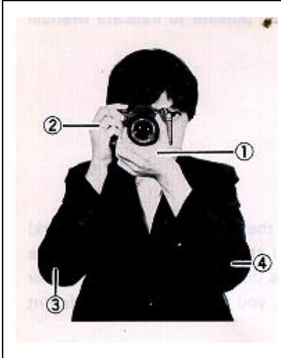
1. The camera should be positioned on the palm of your left hand so that you can use your fingers to turn the Focusing Ring of the lens easily
