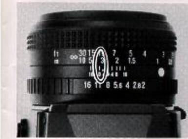
The infrared index mark is an index to correct the focusing point when you use (Black & White film) infrared film and red filters. Since infrared light rays have a longer wave-length than visible light rays, after focusing normally on the subject, you have to set that distance against the infrared index mark.
