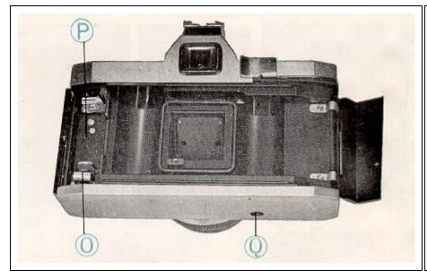
M. Film Wind Lever N. Film Window O. Exposure Meter Battery Housing P. Flash Battery Housing Q. Tripod Screw
