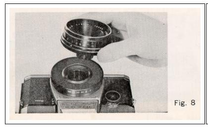
Your camera is equipped with a 55 mm lens which is the proper focal length for general-purpose picture taking. You may also use Rikenon 100mm telephoto or 35mm wide-angle lens.
