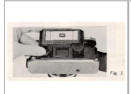
Pull Back Cover Latch (J) and swing open camera back. Place film cartridge in camera upside down as shown in Fig. 1. Close camera and press back cover to snap it shut. Advance Film Wind Lever (M) until number "1" appears in Film Window (N). You need not to make any adjustment for film speed. It is set automatically when film cartridge is seated in the camera.
