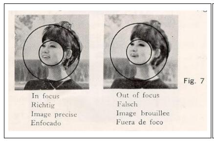
Look into Viewfinder Eyepiece (K) to compose your picture and focus the lens. Rotate Focusing Ring (E) until your subject becomes clear in the micro-prism focusing screen (Fig. 7).
