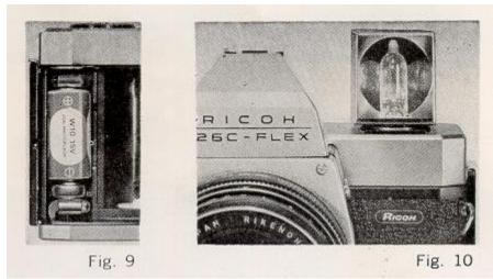
Insert a 15-volt flash battery in Flash Battery Housing (P) according to the (+) ( - ) illustration in the Housing (Fig. 9).
