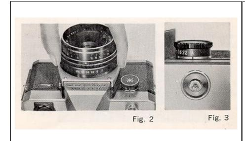
Simply turn Shutter Speed Ring (D) until the desired shutter speed number is set at the red mark (Fig. 2). Be certain the Ring is set at a click stop. "60" (1/60-second) is recommended for subject not in motion. Where motion exists, the faster shutter, 1/125 or 1/300, should be used. When set at "B", the shutter will remain open as long as the Shutter Release Button (A) is depressed.
