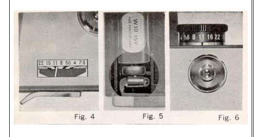
For automatic Turn the Auto/Manual Ring (B) until "A" comes at the black marker (Fig. 3), And the Through-The-Lens CdS exposure meter automatically sets the f-stop always to obtain correct amount of light. The f-stop number at which your picture is taken is shown in Exposure Meter Window (L) on top of camera (Fig. 4).
