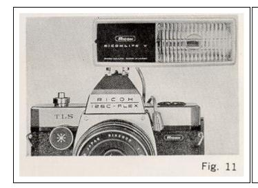
If you are using the normal flash or electronic flash, mount the flash gun onto Accessory Shoe (G) of your camera, and attach the connecting cord to Flash Terminal (I) (Fig. 11). Your camera has a Direct Contact (H) built into Accessory Shoe (G) and cordless type flash guns may be used.
