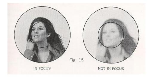
When your subject appears sharpest in the micro-split image, your picture is focused. To take the picture, hold the camera as steady as you can and press Shutter Release Button (C) slowly and smoothly (Fig. 16). Since you are viewing through the lens there is no parallax problem...what you are viewing in the viewfinder will appear in your picture. Even when you shoot close-ups is no danger of accidental cropping.
