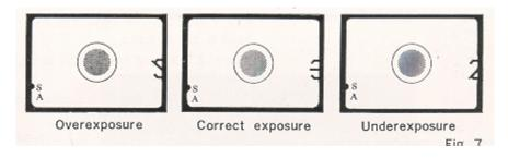
Change the shutter speed to faster speed or use smaller lens opening so that the correct exposure combination is made. If, on the contrary, the exposure meter needle is found under the horizontal position indicating underexposure, you must use a slower shutter speed or bigger lens opening. (Fig. 7)
