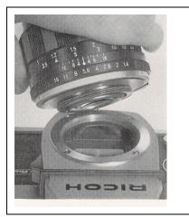
Your camera is equipped with an interchangeable standard lens (Pentax thread mount) which is the proper focal length for general-purpose picture taking. You may also use wideangle lenses for wide angle pictures and telephoto lenses for telescopic picture. To remove the lens continuously turn the lens in a counterclockwise direction until it can be removed. Fig. 20) To insert regular lens or wide angle or telephoto lens, turn lens in a clockwise-direction until lens is secured in position.
