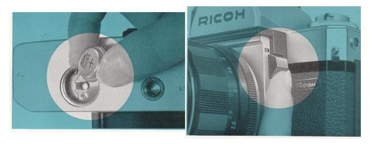
3. Turn "ON" the Exposure Meter Switch (N) pushing it upward. (Fig.5).
