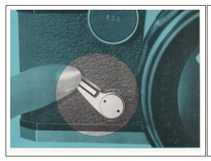
Merely move the self-timer Lever (I) away from the lens (Fig. 19) and press the Shutter Release Button. There will be an 8 second delay before the Self timer will automatically release the shutter and make the exposure for you. Camera should be placed on a tripod or other sturdy support.
