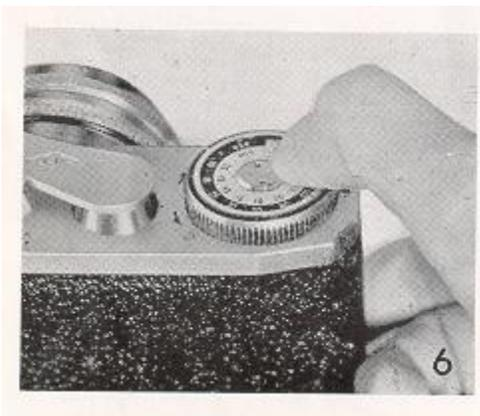
8 ) Bring out the triggermatic-action lever. (See Figure 7 ) You will note that the film counter shows "S" (Start).
