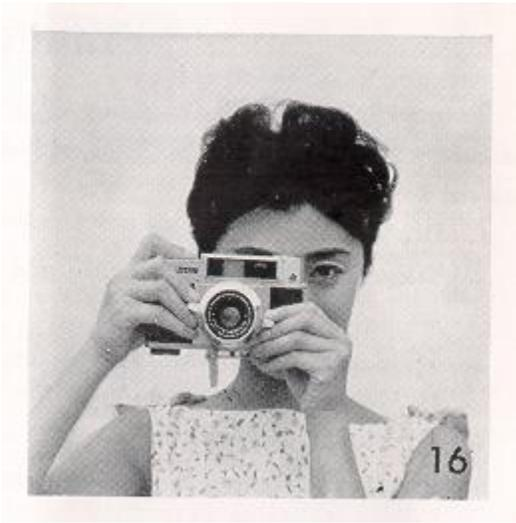
2. Usually the image as seen through the view-and-rangefinder will appear "double" in the center tinted square, which means that the subject is not in focus. When this is the case, move the lever so that the two images merge, or in other words, become superimposed. The subject is now in sharp focus.
