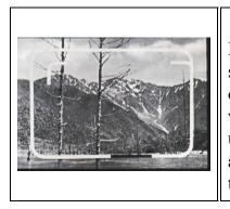
1. Point the camera at the subject to be taken. Look through the BRIGHT FRAME VIEWFINDER and completely frame the subject within the bright frame outline. Any subject within the distance from 5 feet to infinity that can be seen within the frame will be photographed. When taking a photograph at about 5 feet use the inside markings within the bright outline. The marking are corrected for parallax. (Fig. 11) For taking subjects closer than 5 feet, a special close-up adaptor must be attached.
