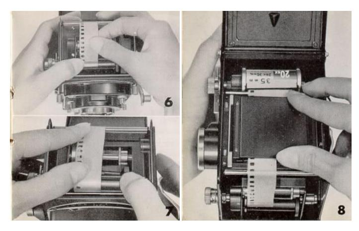
If the Spring is first brought into correct position by turning the Film Take-up Knob this process is made much easier.
