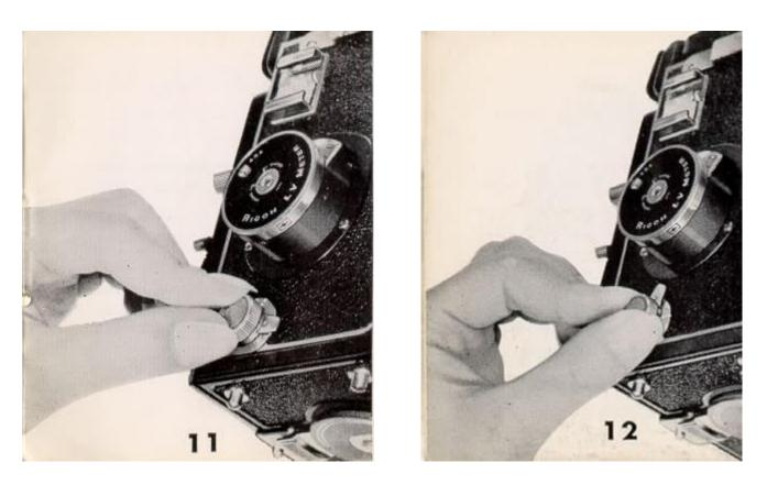
3) In this way, the Knob in depressed position will come to o stop releasing the Auto-stop Mechanism.
