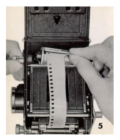
Make sure the 35 mm. Film Cartridge Spool and the Film Rewinding Axle ore properly engaged by turning the Film Rewinding Lever a few times.
