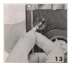
After taking out the exposed cartridge, always match up the Auto-stop Release Lever with the black line and return the Knob to its former position.
