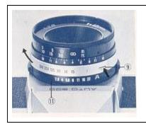
Set shutter speed ring on B (bulb) by depressing bulb setting lever (9). The shutter will remain open as long as the shutter release button is depressed, depending on the length of exposure desired.
