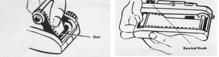
5. Insert film leader into SLOT, pushing film between inside of spool and spring. Be sure film is securely fastened since film will not properly advance if it slips out of slot.
