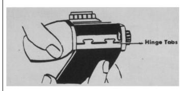
7. Hook HINGE TABS of BACK COVER into slots in HINGE PLATE. Press BACK COVER closed. Lock by sliding RELEASE BAR towards bottom of camera. 6. Pull film cartridge along film track and push cartridge into recess. Push REWIND KNOB in with a slight turning motion.
