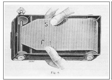
Make sure that all three spool holders as well as the Winding Key are pressed right home then put on the back and lock it, showing the word "closed" (in the manner previously indicated).
