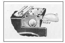
THE VIEW FINDER is normally in the correct position for taking upright pictures; when the Camera is turned for horizontal views, the View Finder must be moved into the corresponding position by swinging it over with the finger (Fig 3). When taking upright pictures ignore subject shown in portion of Finder marked AA, and when taking oblong pictures ignore those portions marked BB (Fig. 3).
