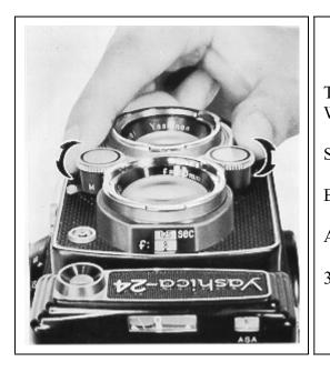
The apertures and the shutter speeds are visible on the Window on the viewing lens. Shutter Speed Scale B. 1, 1/2, 1/4, 1/8, 1/15, 1130, 1/60, 1/125, 1/250 & 1/500 Aperture Scale 3.5, 4, 5.6, 8, 11, 16. 22 & 32
