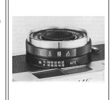
· When using a flashbulb or an electronic flash unit other than the Yashica MS-14DX, select the appropriate lens aperture corresponding to the flash-to-subject distance by referring to the exposure table which comes with the flashbulb or flash unit.
