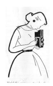
Hold the camera steady, then gently, push the Shutter Release Button.
