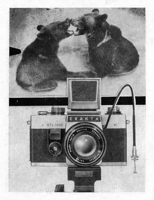
2. The image in any of the viewfinder systems (Finder Hood, Penta Prism, and TTL Penta Prism) will be visible even after the shutter has been released (instant return mirror). The red warning signal in the image in the viewfinder system indicates that the camera is not yet ready for action, and that the rapid-wind lever (9) must be cocked before the shutter is ready for release (See illustration: image seen through the Penta Prism).
