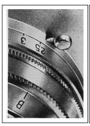
Click Stop for Middle Distance Shot--- enables photographers to take snapshots of middle -distant objects from 6 ft. to 15 ft. at aperture of f/8 without focusing.
