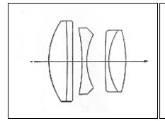
"HIGHKOR" LENS is designed for miniature negatives which are to be enlarged to huge proportions and yet are to retain in the completeness of the minutest detail. They are coated to reduce surface and internal reflections.
