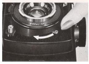
When using the self-timer, always see to it that the Flash Synchronizer Selector is switched to "X" position
