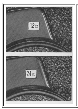
When the back cover is closed, the exposure load reminder window will show "12 EX" (green) in case of 120 film, and "24 EX" (red) in case of 220 film, to check the exposure load of the film in use.
