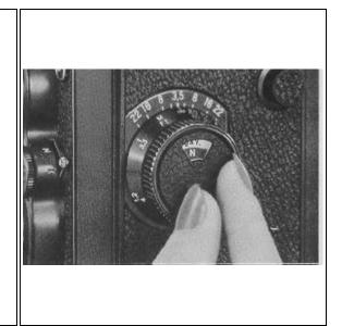
After loaded the film, turn the Film Type Indicator as illustrated, so that the letters equivalent to the film type in use are indicated in the window.
