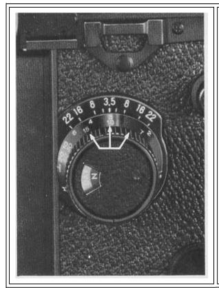
The depth of field for a given aperture and camerato-subject distance can be read off the depth-of-field scale around the Focusing Knob. By checking this scale, you can easily determine before shooting the extent over which the objects will appear sharp and clear.
