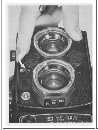
Turn the Aperture Control Dial and coincide the yellow follower needle (coupled to the aperture mechanism) with the red meter pointer (coupled to the shutter mechanism), both visible in the Exposure Indicator Window.
