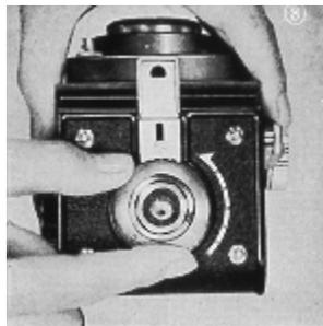
(7) Advance the film by slowly winding the Crank until the arrow on the film points to the triangles on either side of the camera body.
