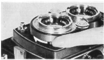
For taking self-portraits or group pictures, you have about 8 seconds to get into the picture. Therefore your camera must be mounted on a tripod or brace to prevent a blurred picture.
