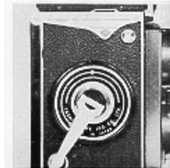
The shutter should not be kept wound when not in use because it weakens the shutter spring, and there is the possibility you may unknowingly press the shutter button and waste a film.
