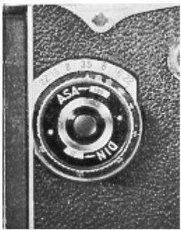
The ASA speed dial on the focusing knob is to keep record of your film speed. Turn dial to your film speed number. Since the camera has no meter, this is just to remind you what film you have in the camera.
