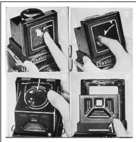
(A) Raise the Magnifying Glass by pressing the front of the Focusing Hood Cover inward, holding the Focusing Hood so that it does not close.
